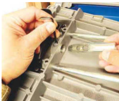
With the table removed the sleeve can be swapped for different drill sizes
